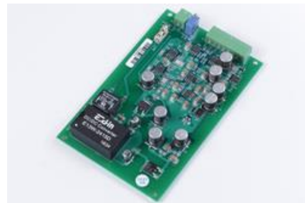
Load cell 放大器(General purpose) Model: LCA-9K-G1000
